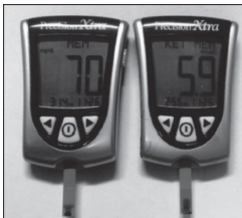
Photo 9.2. Two monitors are set up to test blood glucose and betahydroxybutyrate from the same finger prick.
