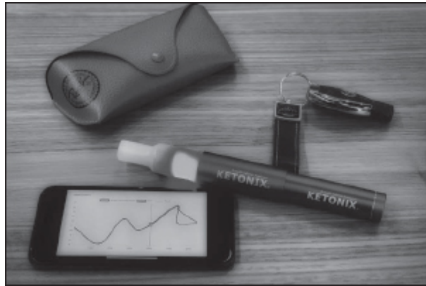
Photo 9.3. A breath analyzer can be used repeatedly throughout the day to detect acetone and can be used to estimate blood ketone levels.
